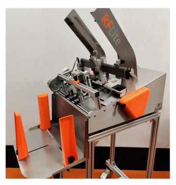
The RF Lite carton feeder would enable the production team to print batch codes on all sizes of cartons - from 30 x 70mm up to 300 x 200mm. This meant that even their smallest size carton could be fed through the system at up to 300 per minute, extending to 400 per minute for larger sizes. And changing from one carton size to another takes only a few seconds, avoiding any delays in throughput.
