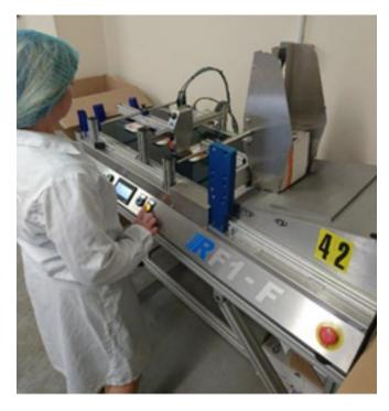
On the RF1 system, because the cartons are deposited onto a conveyor belt on a horizontal bed for printing, the code can be placed anywhere. This contrasts with rival systems on which the carton is fed down the front of the machine and gripped in a side belt - a configuration that limits code placement options. The RF1 system also offers users the flexibility to print cartons flaps-leading or body-leading, enabling printing along the length of the carton.
