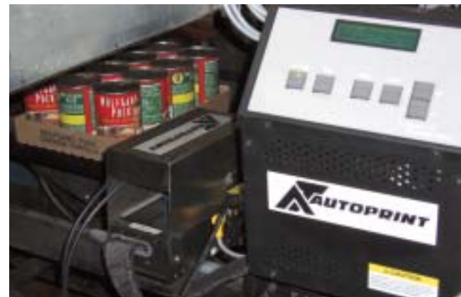
Within the tray packer at Faribault Foods is the print head housing that holds three HP thermal inkjet cartridges. It is immediately left of the controller for the AUTOPRINT® coding system. A case, moving to the right, has just received a code and is moving toward a bundling station.
