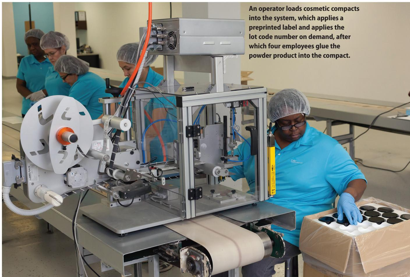
An operator loads cosmetic compacts into the system, which applies a preprinted label and applies the lot code number on demand, after which four employees glue the powder product into the compact.
