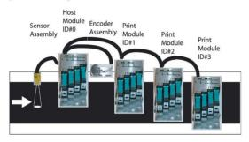
The host print module interface can be accessed from the system PC using either a USB or Ethernet communication port. It is easy to connect multiple print modules to build a taller message or to configure systems for opposite side and adjacent side printing. This can be done with standard connection cables or with custom cables up to 20 feet long.
