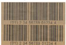
**384Jet** @ 100 FPM 6mm gap, 40% decode-ability (just above 'C') Print contrast 37 'D'
