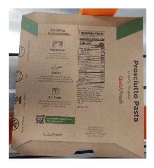
they could create a carton that was semi-generic and then we could just add the different fields for the variable information that needed to be printed. We needed a high-res mark because they have the nutrition facts on there. And to get that smaller print, be able to read it, and fit it on the carton, we needed a high-resolution type of printer."
